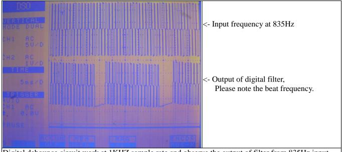
Digital debounce circuit work at 1KHZ sample rate and observe the output of filter from 835Hz input
