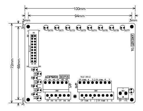
4.3 JS51053 for CN1/CN2 20PM Din rail mounted dummy wiring board
